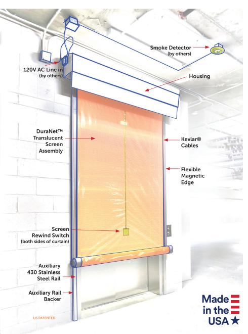
**Rewind Switch.** The Smoke Guard system screen rewind switch may be activated from both sides of the screen. This feature allows elevator occupants to exit from the elevator car using the interior (shaft side) of the switch. The screen will then redeploy after egress, as long as the smoke detector continues to be activated. In the event of power outage, the vertical edge of the curtain can be pushed away from the rail to allow passage with a force less than 15 lbs. as referenced by the ICC.
