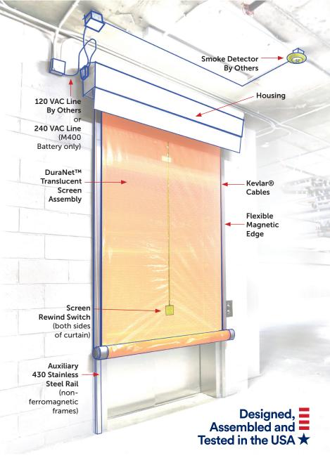
Rewind Switch. The Smoke Guard system screen rewind switch may be activated from both sides of the screen. This feature allows elevator occupants to exit from the elevator car using the interior (shaft side) of the switch. The screen will then redeploy after egress, as long as the smoke detector continues to be activated. In the event of power outage, the vertical edge of the curtain can be pushed away from the rail to allow passage with a force less than 15 lbs., as required by the IBC.
