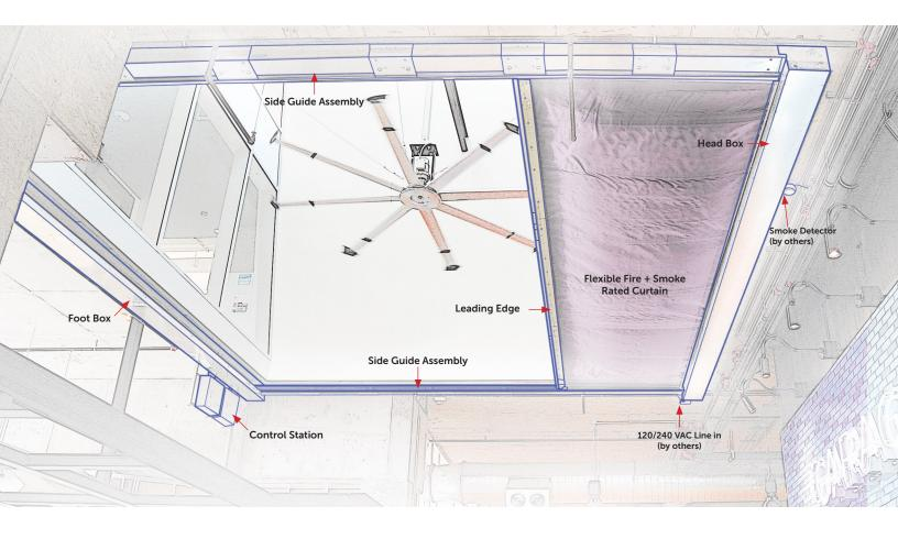
**System Operation.** The system is deployed upon a signal from the local smoke detection system or a smoke control panel. System power requirement is 120/240 VAC. The unit is also equipped with a 24 VDC battery back-up system that is maintained by the electronic controls. When required the system can also be connected to building standby power. The controls include a universal power supply that supports 120/240 VAC operation.
