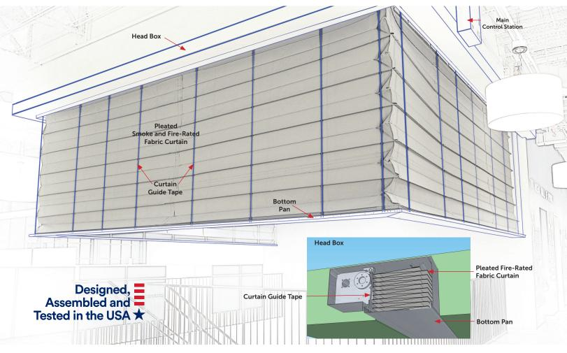
**System Operation.** The system is deployed upon a signal from the local smoke detection system or a smoke control panel. System requires 120/240 VAC power. The unit is also equipped with a 24 VDC battery back-up system that maintains the electronic controls. When required the system can be connected to building standby power. The controls include a universal power supply that supports either 120/240 VAC operation.
