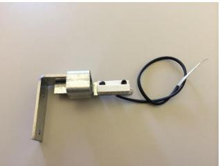
uplimit switch assembly (w/ magnetic target, not shown)
