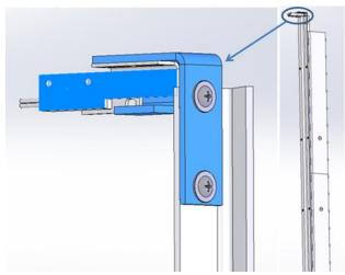
After the Bottom Bar Assembly is complete (as described in the next section), attach the Magnetic Target to the bottom bar as shown below, using the peel and stick adhesive <u>AND</u> #6 self-tapping screws. The target must be centered, side-to-side, with the Up Limit Switch assembly. No vertical adjustment is necessary.
